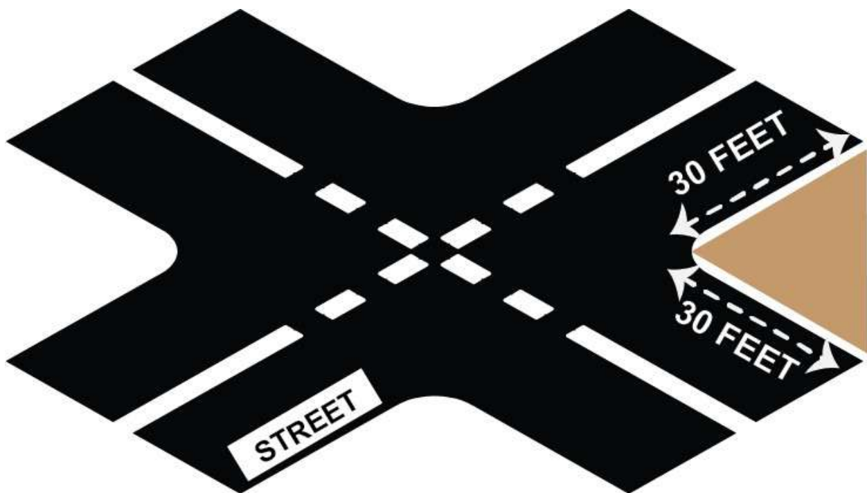
Figure 4.10.2-A. Unsignalized Intersection Vision Clearance Triangle
